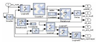
Fig 3. Control logic block for the first layer
