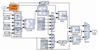
Fig. 7. The hardware architecture of the PLAN approximation of sigmoid function
