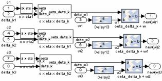
Fig. 9 Hardware implementation of the weights calculus block
