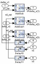
Fig. 13 Hardware implementation of the changed weights
