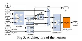
For implementation in FPGA of the activation function was used the PLAN approximation (<u>Piecewise Linear Approximation of a Nonlinear</u> function), proposed by Amin, Curtis and Hayes–Gill [7]. The PLAN approximation uses digital gates to directly transform from x to y. The approximation of the sigmoid function is presented in Table 1. The calculations need only be performed on the absolute value of the input x.
