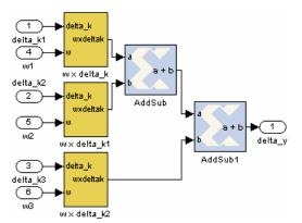
Fig. 11 Hardware implementation of the Delta\_y calculus block
