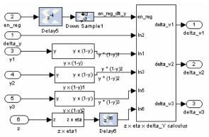
Fig. 12 Hardware implementation of the Delta\_v calculus block
