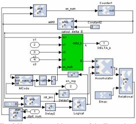
Fig. 8 Hardware architecture of the Error check block
